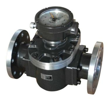
Special Note: If fitting this register to a meter that had a "M", "MI", or "MR" register previously fitted, the meter will need to be rotated 180° to the flow that it was previously installed. Original install → Flow Left to Right as per arrow marking pointing to the right, once the new register is installed the flow should be ← Left to Right but the arrow pointing left.
