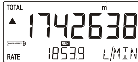
Fig. 4: Example of low-battery alarm.
