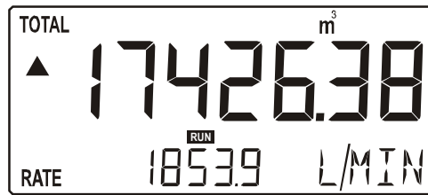
Fig. 3: Example of display information during process.
