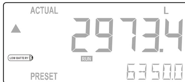
Fig. 6: Example of low-battery alarm.
