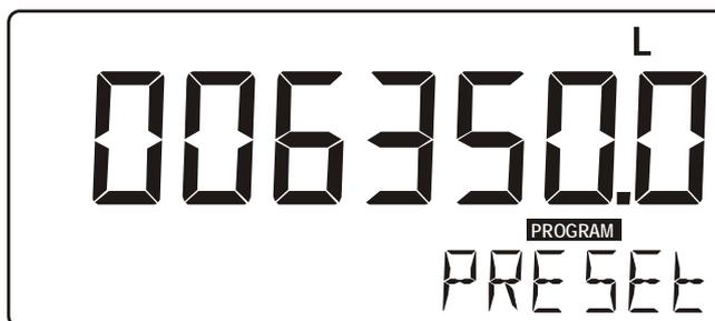
Fig. 3: Example display information during programming preset value.
