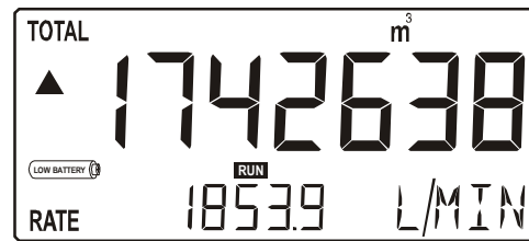
Fig. 4: Example of low-battery alarm.
