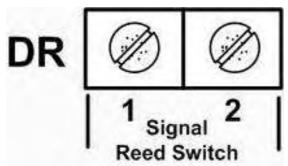
The DR unit cam only accept a reed switch input, this sensor has been selected as the most common sensor and requires very little power with small effect on battery life.
