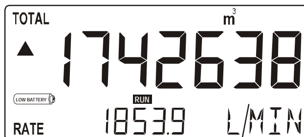
Fig. 4: Example of low-battery alarm.
